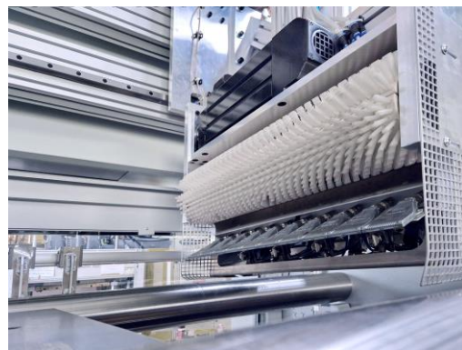
Brush module with spraying device
